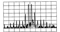
Figure 1-Worst-case spectral display of the Yaesu FT-840 transmitter during twotone intermodulation distortion (IMD) testing. Worst-case third-order product is approximately 28 dB below PEP output, and the fifth-order product is approximately 49 dB down. Vertical divisions are 10 dB; horizontal divisions are 2 kHz. The transceiver was being operated at 100 W PEP output at 14 MHz.
