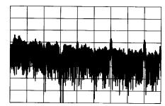
Figure 5—Spectral display of the S & S Engineering ARK 40 transmitter output during composite-noise testing. Power output is 3.6 W at 7 MHz. Vertical divisions are 10 dB; horizontal divisions are 2 kHz. The log reference level (the top horizontal line on the scale) represents 60 dBc/Hz and the baseline is 140 dBc/Hz. The carrier, off the left edge of the photograph, is not shown. This plot shows composite transmitted noise 2 to 20 kHz from the carrier.
