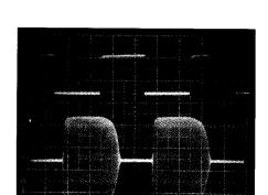
Figure 4—CW-keying waveform for the S & S Engineering ARK 40. The upper trace is the actual key closure; the lower trace is the RF envelope. Horizontal divisions are 10 ms. The transceiver was being operated at 5 W output at 7 MHz.
